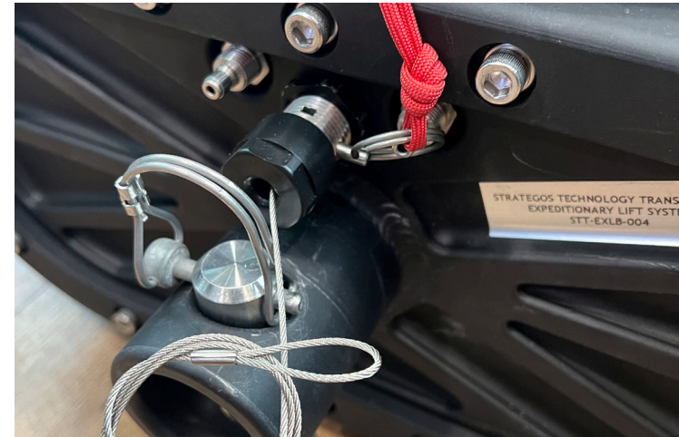
Pin and Lanyard Properly Rigged
