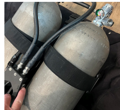
Pointing to bleed valve
