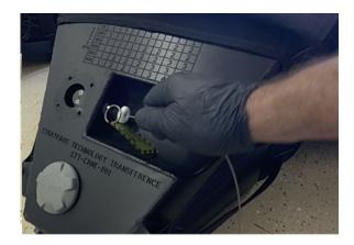
13.4.1. Test pull the Manual Pull Lanyard against the safety pin. Manual Pull Lanyard should not be able to be pulled free.
