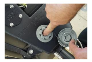
14.3. Thread the EIDV valve adapter hose onto EIDV valve.
