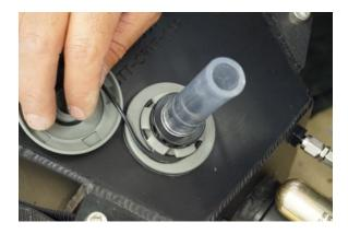
14.4. Hook adapter hose up to foot pump or shop air line on the inflation port.
